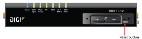
Press and hold the **Reset** button for **5** seconds. The device reboots automatically. The device reset to factory defaults. Follow the instructions in the *Digi LR54 Quick Start Guide* to reconfigure the device.
