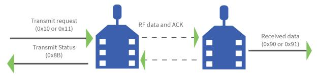
Use the **AP** command to choose the type of data frame you want to receive, either a (0x90) RX Indicator frame or a (0x91) Explicit Rx Indicator frame.
