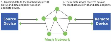
4. Source receives loopback transmission and sends received packet out the UART.
